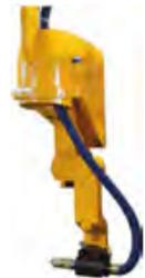
3D rotator with a tilt range up to  $120^\circ$  and Z-axis stroke up to 1,500 mm enables cutting of 3D shapes such as open profiles I, H, U or L and domes.
