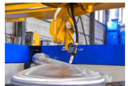
The pantograph plasma rotator with a tilt up to 120° enables weld edge preparation also on the bottom edge of a dome.
