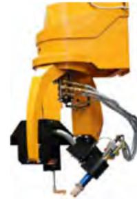
5-axis rotary bevel head with endless rotation enables oxyfuel bevel cutting of plates, pipes and profiles up to  $65^\circ$ . The innovative ITH torch holder includes sensors for torch displacement detection, IHS and auto-calibration.
