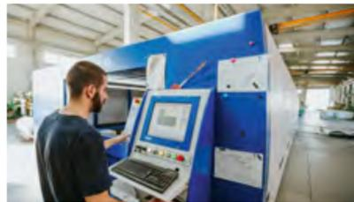
Faddikorr opted for two CNC cutting machines from MicroStep: fiber laser machine MSF with a straight tool station, with work area 6,000 x 2,000 mm (below), and a sturdy 3D plasma cutter DRM equipped with a pantographic plasma rotator capable of tilting up to 120° designed solely for cutting of domes up to Ø 3,500 mm (on top).
