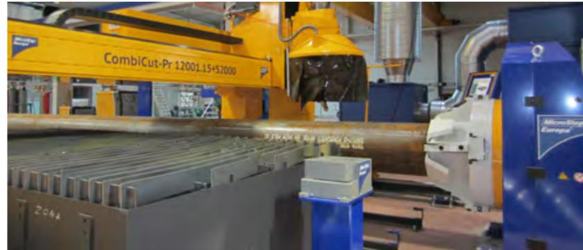
ables bevel cutting up to 50° on both plates and pipes. "We used to buy pipes from a supplier. The problem was that it was very inflexible – deliveries took too long," says Pierre Ruble.
