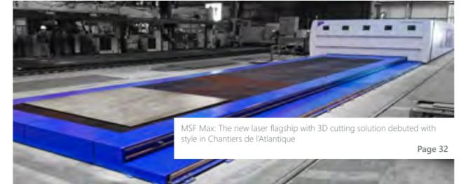
MSF Max: The new laser flagship with 3D cutting solution debuted with style in Chantiers de l'Atlantique
