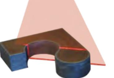
Laser scanner dedicated for scanning of both the contour and position of a straight pre-cut part in ABP feature – additional cutting of bevels for weld edge preparation. ABP technology is available for plasma, laser, oxyfuel and waterjet cutting technologies.
