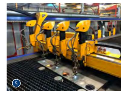
One of the four cutting gantries at Doppelmayr is equipped with four oxyfuel cutting heads for cutting of big material thicknesses. The more than 60-meter-long production line runs in three shifts at the headquarters of the company in Wolfurt (Austria) near the Bodensee Lake.
