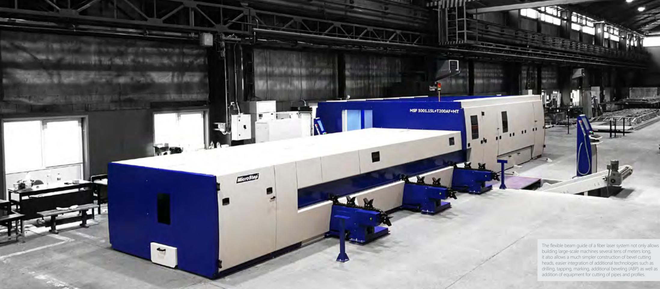
The flexible beam guide of a fiber laser system not only allows building large-scale machines several tens of meters long, it also allows a much simpler construction of bevel cutting heads, easier integration of additional technologies such as drilling, tapping, marking, additional beveling (ABP) as well as addition of equipment for cutting of pipes and profiles.
