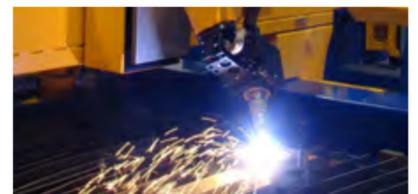
With rotator from MicroStep, V-, Y-, and (under certain conditions) also X- and K-cuts can be produced additionally on already pre-cut parts.
