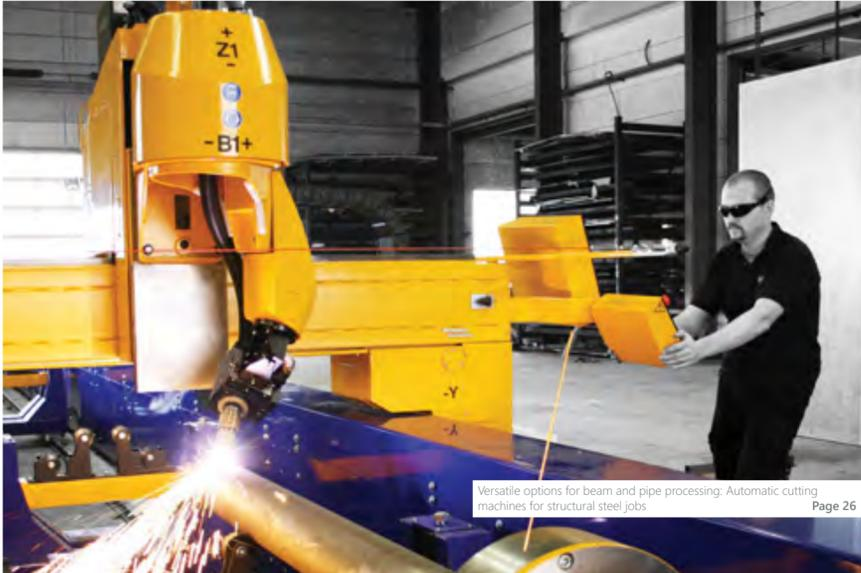
Versatile options for beam and pipe processing: Automatic cutting machines for structural steel jobs
