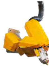
Laser bevel cutting head with tilting ability up to  $45^\circ$  for fiber laser cutting of various types of materials.
