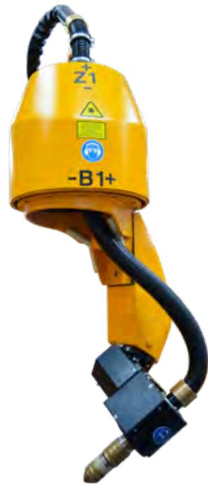
5-axis rotary bevel head with endless rotation enables plasma bevel cutting of plates, pipes, profiles and domes up to  $52^\circ$ . The innovative ITH torch holder includes sensors for torch displacement detection, IHS and auto-calibration.
