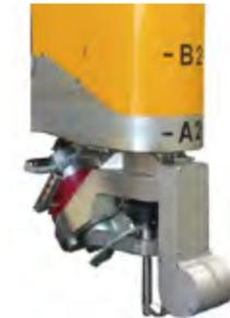
5-axis rotary bevel head for waterjet enables bevel cutting of all types of materials up to  $45^\circ$ . Adaptive taper compensation (ABC) and periodic height sensing (PHS) are included by default.
