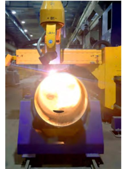
Top left + right: Gree's combined pipe & dome cutting machine PipeCut allows to cut pipes up to Ø 610 mm and a length of 12 m as well as domes up to Ø 1,200 mm. Bottom left: Gree Electric Appliances Inc. was chosen to participate on prestigious projects such as the National Stadium (Soccer City) in South Africa's Johannesburg.
