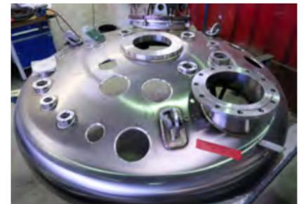
GEA Production Kitzingen opted for a multi-functional MG machine that allows to process metal sheets as well as dished ends.
