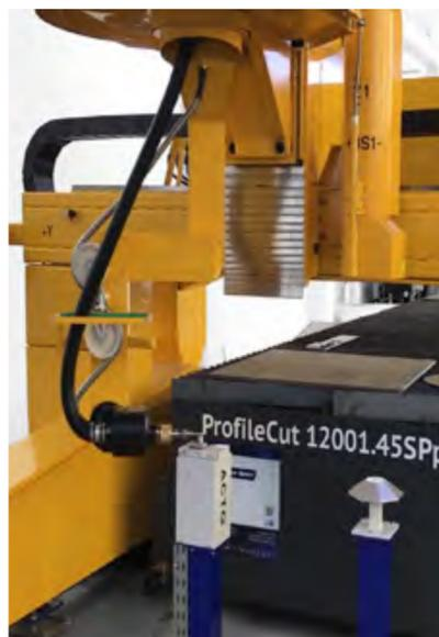
Apart from standard flat-bed machines, MicroStep offers an exceptional variety of equipment for processing of 3D rotary objects and structural steel sections of various shapes. The rotary objects include differently sized circular, square and rectangular hollow sections (diameters of circular sections reach from Ø 30 mm up to Ø 2,000 mm), conical pipes, torispherical or elliptical domes and elbows.
