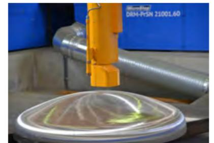
The laser scanner can reach the entire dome surface. The measured data are compared with the ideal dimensions on which the cutting plan is based and deviations are automatically compensated for during the cutting process.
