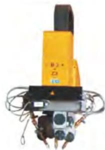
Oxyfuel triple torch with fully automatic gas console enables bevel cutting of V-, X-, Y- and K-cuts with 3 oxy torches within bevel range  $20^\circ - 50^\circ$ . Tilting angle and span of torches can be set manually or automatically.
