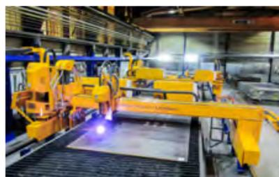
In order to renew its machine park and to become faster and more flexible in production, the Baden-Württemberg based company MAP Prinzing Brennschneidtechnik GmbH was looking for new cutting machinery. The job cutting business found their solution at MicroStep – and invested into a complex CombiCut machine. This multi-functional system enables bevel cutting with plasma, 2D oxyfuel cutting, drilling, tapping, countersinking and marking with a powerful combination of two gantries.
