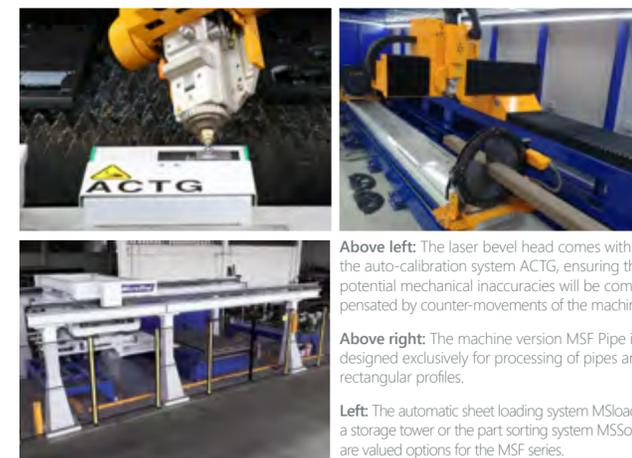
Above left: The laser bevel head comes with the auto-calibration system ACTG, ensuring that potential mechanical inaccuracies will be compensated by counter-movements of the machine.
