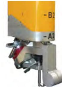
5-axis rotary bevel head for waterjet enables bevel cutting of all types of materials up to  $45^\circ$ . Adaptive taper compensation (ABC) and periodic height sensing (PHS) are included by default.
