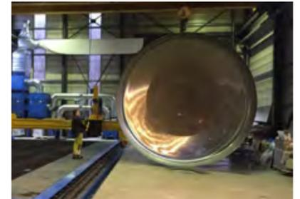
When designing the plasma cutting machine, the focus was on the precise and flexible processing of domes. A special dome cutting table supports domes from 500 mm up to 5,500 mm in diameter.
