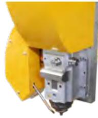
Laser tool station for fiber laser 2D cutting.
