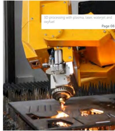
3D processing with plasma, laser, waterjet and oxyfuel
