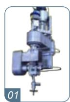
5-axis rotation head for waterjet cutting enables fully automatic bevel cutting of conductive and non-conductive materials with bevel up to 45°.
