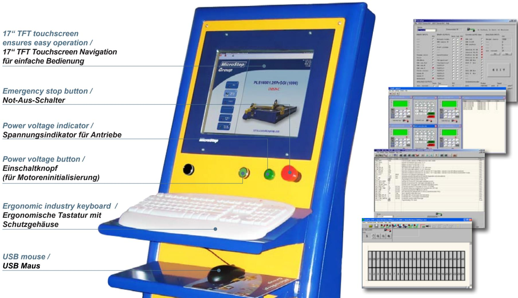
Integrated parameter databases for different technologies ensure high efficiency and stable quality of cuts, interactive elements with bubble help allow real-time control of the machine. Machine can be comfortably integrated into company's workflow with a range of Intranet applications and accessed via SQL databases and web services. Advanced Remote diagnostics tools ensure fast and cost-saving maintenance of the system via internet.
