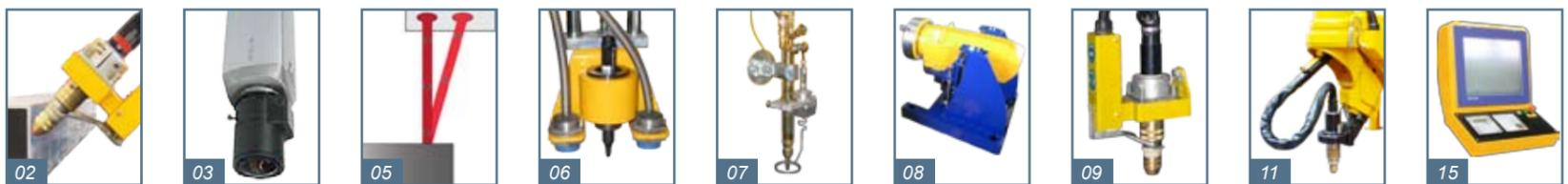
Machines from the PipeCutter series can be equipped with following additional devices: 02. Tilting, 03. CCD camera, 05. Laser sensor, 06. Marking, 07. Oxyfuel, 08. Pipe cutting device, 09. Plasma, 11. Rotator, 15. Touch Screen
